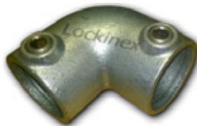
A06-8 90 degree elbow joint. Used for forming 'D' ends to terminate a run of handrail & turning rails at corners.
