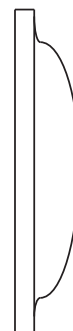
This cover plate is suitable only for the HB1RS, HB3RS and HB3FS type handrail brackets.
