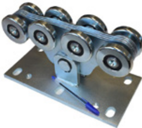
8 Wheeled Carrier. SLGHW-15 Recommended Max load of 1000kg. Wheel Dia = 70mm Nominal .
